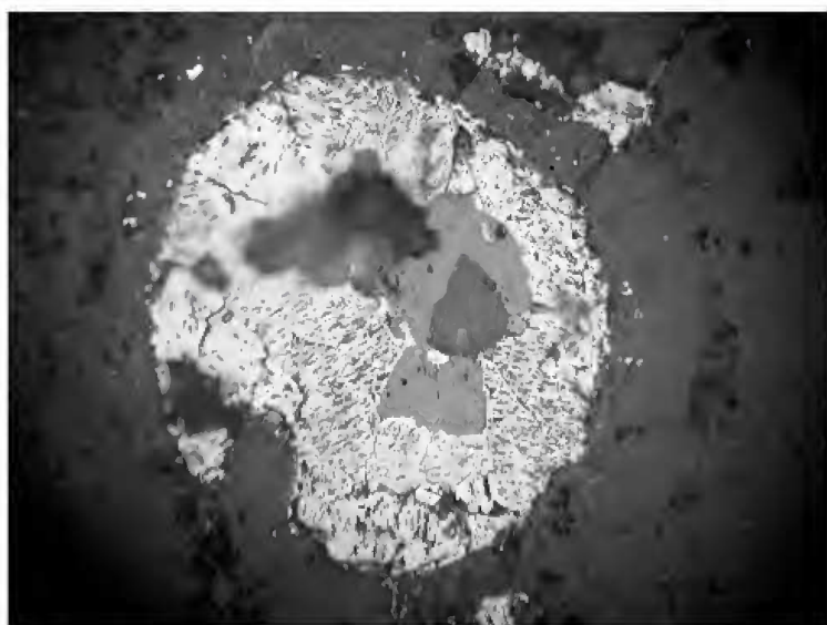
Fig.13- Reflected light photomicrography showing a troilite grain in a spheroidal shape with silicate inclusions, resembling a metallic chondrule. Length of field 0.7mm.
